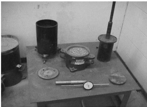
*Figura 57.* Ensayo mesa vibratoria ASTM D4253.
