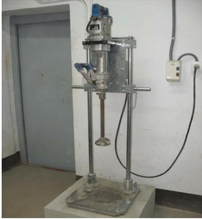
*Figura 37.* Martillo Vibratorio ASTM D-4253.
