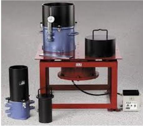
Figura 36. Mesa vibratoria ASTM D-4253.
