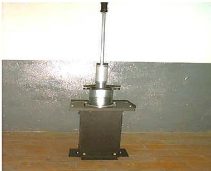
Figura 32. Martillo Marshall ASTM D-1559.
